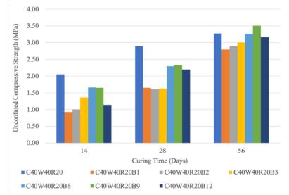
Figure 1 UCS development of composite clay liner containing various amounts of bentonite
