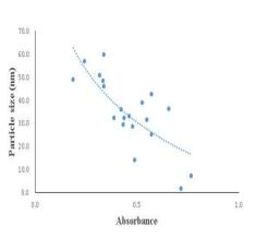
**Figure 9.** Relationship between the size of AgNPs and peak absorbance in UV-vis spectra.
