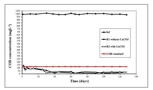
Figure 6 Influent and effluent concentration of COD in SBR1 and SBR2.
