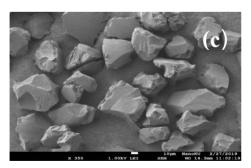
Figure 2 The FE-SEM of the adsorbents. The scale bar represents 100 nm, (a) Fe<sub>3</sub>O<sub>4</sub> magnetite nanoparticles (MNPs); (b) GCB; (c) PSA
