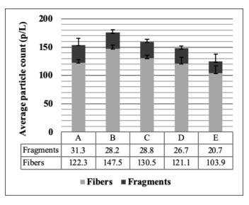
**Figure 5** Average particle count for 6.5-20 µm (Fluorescent tagging)
