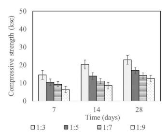
Figure 2 Compressive strength of original interlocking blocks
