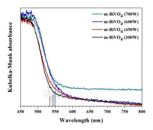
**Figure 4.** UV-vis DRS spectra of the m-BiVO<sub>4</sub> powders synthesized at different microwave powers.
