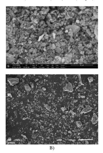
Figure 1 SEM images of (A) LS and (B) BA.
