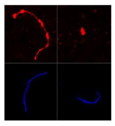
Figure 3 Fluoresced particles found in bottled water samples
