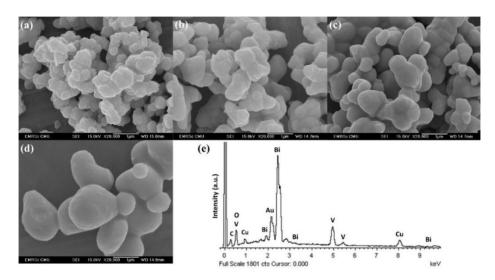
Figure 3. FESEM images of the m-BiVO<sub>4</sub> powders synthesized at (a) 300,
