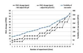
Figure 3 Optimum PACL dosage from jar test at varying raw water turbidity
