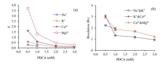
**Figure 5** The performance of metal ion separation using different concentrations of PDCA. The data represent: a) k' and (b) resolution (Rs). The experimental condition is the same as described in Figure 4.
