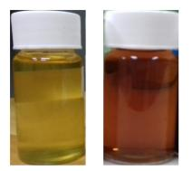
Figure 1. Orange peel extract (left)andbiosynthesizedAgNPssuspension (right).
