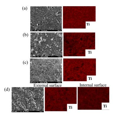
**Figure 3** SEM and EDX mapping images of TiO<sub>2</sub> samples (a) External surface of PE-TiO<sub>2</sub> pellets, (b) External surface of CT 50 pellets, (c) External surface of CT40 pellets and (d) External and internal surface of CT30 pellets.
