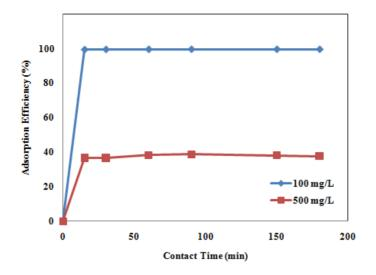
Figure 8 Influence of contact time on the Basic Red 29 adsorption onto MAC at 30<sup>o</sup>C (pH, 8; adsorbent dose, 100 mg)
