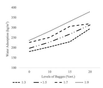
Figure 5 Water adsorption of original interlocking blocks.
