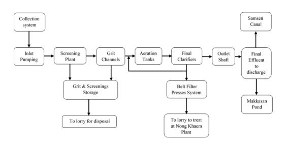
Figure 1 Flow chart of Din Daeng wastewater treatment plant
