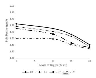
Figure 4 Bulk density of modified interlocking blocks.
