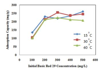
Figure 9 Influence of initial Basic Red 29 concentration and temperature on the Basic Red 29 adsorption onto MAC (pH, 8; adsorbent dose, 100 mg)
