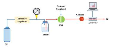
**Figure 1** Schematic diagram of the OTIC system; NC=nitrogen gas cylinder, INJ= 2-position-6-ports-injection valve, W=waste.
