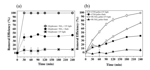
**Figure 4** Degradation of glyphosate under dark and UV conditions (a) TiO<sub>2</sub> powder and (b) clay TiO<sub>2</sub> pellets and PE-TiO<sub>2</sub> pellets
