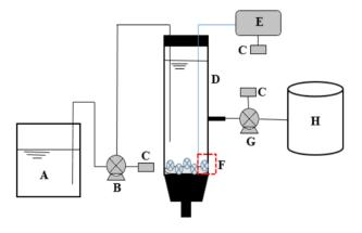
**Figure 1** experiment set-up: (A) Influent tank; (B) Influent pump; (C) Timer; (D) Reactor; (E) Air pump; (F) Air diffuser; (G) Effluent pump; (H) Effluent tank
