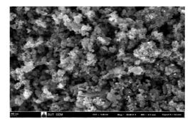
Figure 1 FE-SEM image of Carbon black 20000 kx
