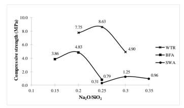
Figure 1 Strength of geopolymer at various  $Na_2O/SiO_2$
