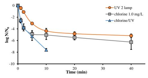
Figure 4 TRB inactivation by chlorination, UV irradiation and chlorine/UV process (n = 3)
