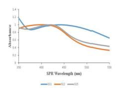
**Figure 4.** Effect of pH on absorbance spectra of biosynthesized AgNPs.
