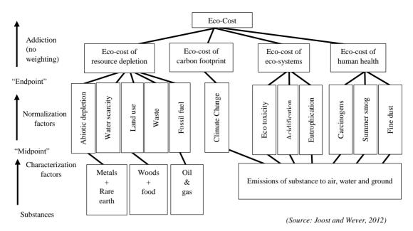
Figure 4 Calculation structure of the system of Eco-costs 2012 result
