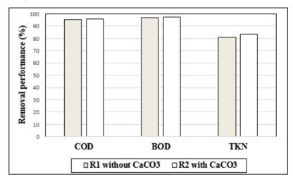
Figure 10 Overall of removal performance in reactor SBR1 and SBR.
