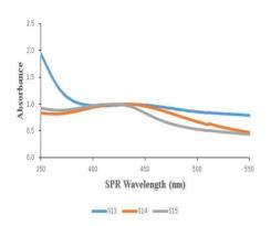
**Figure 5.** Effect of AgNO3 concentration on absorbance spectra of biosynthesized AgNPs.
