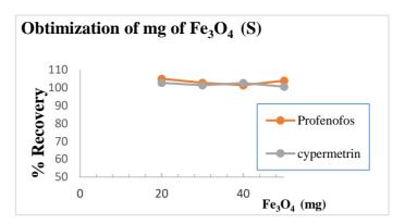
**Figure 4** Effect of mass of Fe<sub>3</sub>O<sub>4</sub> on the extraction efficiency of profenofos and cypermethrin (5 mg/ kg).
