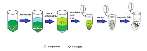
Figure 1 Schematic of developed sample preparation.  $Fe_3O_4$  magnetic nanoparticles ( $Fe_3O_4$  MNPs); graphitised carbon black (GCB); primary secondary amine (PSA)
