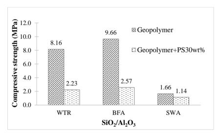
Figure 3 Strength of geopolymer with/without 30 wt.%PS,
