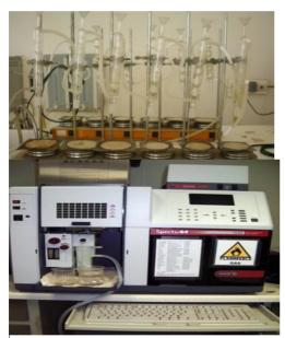
Figure 5: Atomic Absorption Spectrophotometer (AAS)
