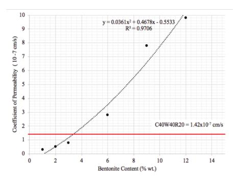
Figure 2 Coefficient of permeability of compacted clay and wastes.
