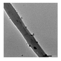
Figure 2 TEM image of PLA/PVP/GO nanofiber filaments
