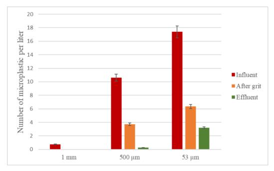
Figure 2 Number of microplastic found in each stage of WWTP
