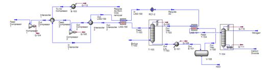
Figure 3. Schematic of the cryogenic CO<sub>2</sub> separation system
