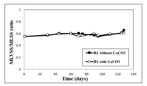
Figure 5 MLVSS/MLSS ratios in SBR1 and SBR2 during 128 days of operation.
