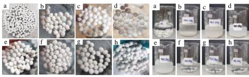
**Figure 1** (A) The appearance and (B) the stability of TiO<sub>2</sub> pellets in water by observed the turbidity (a) PE-TiO<sub>2</sub> pellets, (b) CT0 pellets, (c) CT5 pellets, (d) CT10 pellets, (e) CT20 pellets, (f) CT30 pellets, (g) CT40 pellets and (h) CT50 pellets
