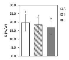
Figure 3 Phosphorus accumulation in sludge. SRT 20 days (A); SRT 25 days (B); SRT 60 days (C). Different superscript letters (a) are significant differences (p < 0.05)
