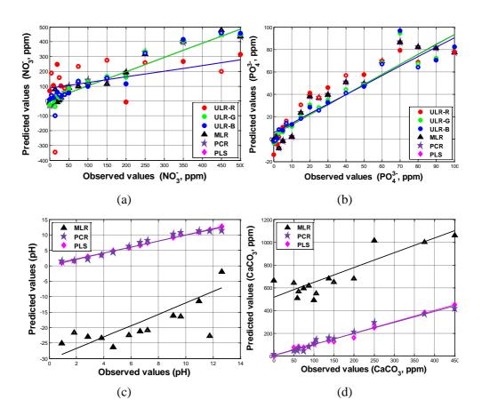
**Figure 2** Correlation graphs between expected and predicted of (a)  $NO_3^-$ , (b)  $PO_4^{3-}$ , (c) pH and (d) total hardness. Training and test samples were labeled using opened and closed face symbols, respectively.
