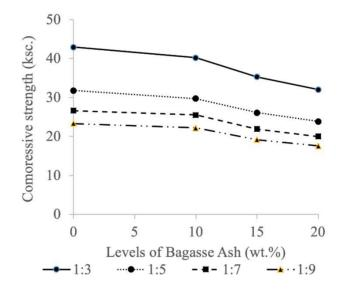
Figure 3 Compressive strength of modified interlocking blocks.
