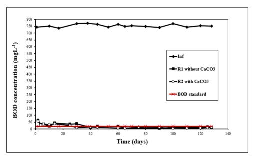
Figure 7 Influent and effluent concentration of BOD in SBR1 and SBR2.
