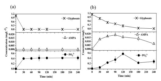
**Figure 5** Concentration of glyphosate and its byproducts during photocatalytic degradation (a) TiO<sub>2</sub> powder and (b) CT30 pellets
