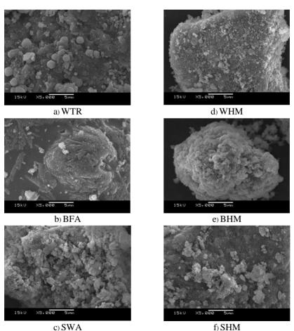
**Figure 6** SEM–EDS images of of geopolymer with and without 30 wt.% PS at SiO<sub>2</sub>/Al<sub>2</sub>O<sub>3</sub> ratio of 3:1
