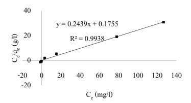
Figure 6 Langmuir adsorption isotherm of Cr
