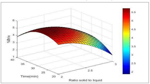
**Figure 5** The 3D-graph showing the effect of treatment time and 1:15 solid to solvent ratio on %brix at 0.55% wt concentration of solution
