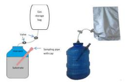
Figure 1 Schematic drawing of the experimental digester with aluminum film gas storage bag 2.3 Analytical methods
