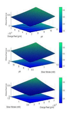
**Figure 6.** Surface plots showing absorbance as a function of orange peel conentration and pH (top), AgNO<sub>3</sub> concentration and pH (middle), and orange peel extract concentration and AgNO<sub>3</sub> concentration (bottom).
