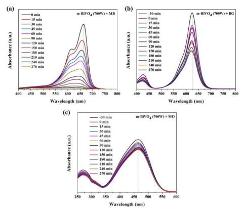
Figure 6. UV-vis absorption spectra changes of (a) MB, (b) BG, and (c) MO aqueous solutions as a function of the reaction time.
