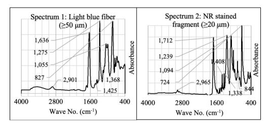
Figure 7: ATR-FT-MIR spectra of a fiber and fragment detected as PET
