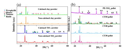
**Figure 2** XRD diffraction patterns of the  $TiO_2$  samples (a)  $TiO_2$  powder and white clay and (b) PE-TiO<sub>2</sub> pellets and clay  $TiO_2$  pellets
