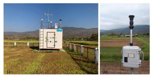
Figure 1 Sampling site (a) Mae Hia AQM station and (b) mini volume air sampler.
