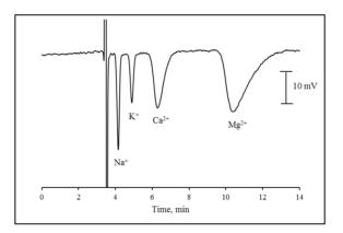
**Figure 3** Chromatograms of alkali and alkaline earth metal with 1 mM PDCA as an eluent for mixed cation (111  $\mu$ M Na<sup>+</sup>, 78  $\mu$ M K<sup>+</sup>, 117  $\mu$ M Ca<sup>2+</sup>, and 316  $\mu$ M Mg<sup>2+</sup>) with 25 nL injected. Column 1.3 m x 50  $\mu$ m, 13 layers of PBMA polymer, eluent 1 mM PDCA, flow rate 0.7  $\mu$ L/min, using a commercial C4D detector.
