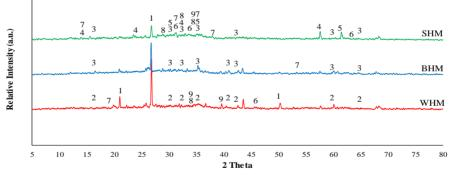
Figure 5 XRD of geopolymer with 30 wt.%PS,
