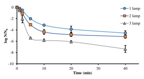
**Figure 3** TRB inactivation by UV irradiation (n = 3)
