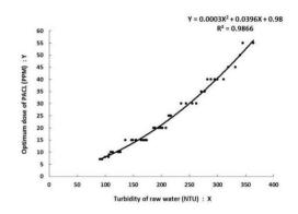
**Figure 4** The relationship between turbidity of raw water (X) and optimum dose of PACL (Y)
