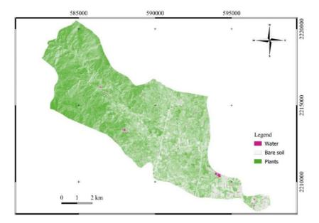
Figure 4 Transformed image, based on Thaichote image, derived from NDVI
