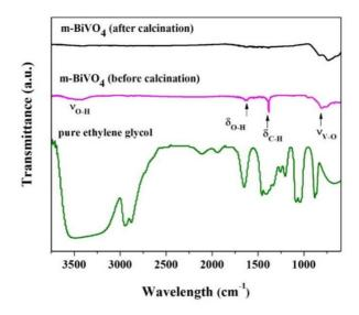
**Figure 2.** FTIR spectrum of the m-BiVO<sub>4</sub> (700 W) powders before and after calcination.
