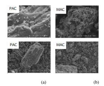
Figure 3 Scanning electron microscopy images of PAC and MAC at different magnifications
