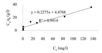
Figure 5 Langmuir adsorption isotherm of Ni
