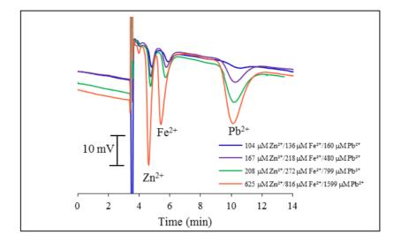
**Figure 6** Chromatogram of standard transition metal. Column 1.3 m x 50  $\mu$ m, 13 layers of PBMA, eluent 2 mM tartaric acid/1 mM oxalic acid, flow rate 0.7  $\mu$ L/min, commercial C4D detector, injection volume 24 nL.
