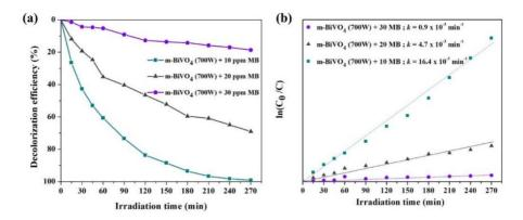
**Figure 7.** (a) %DE and (b) photocatalytic reaction kinetics of the m-BiVO<sub>4</sub> (700 W) photocatalyst for the photodegradation of MB with different initial dye concentrations.
