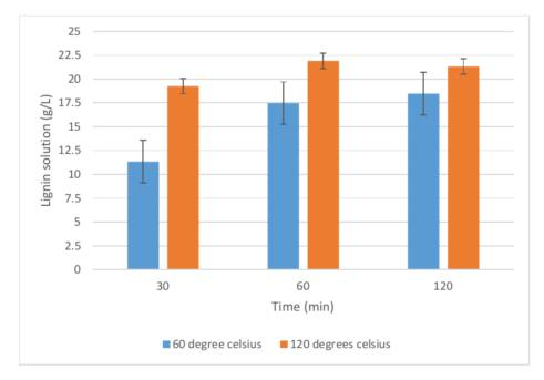
Figure 3 The amount of lignin solution from temperature and time study.
