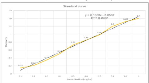
**Figure 6** Calibration curve for determination of reducing sugar in extract of water hyacinth by MAE method using UV-Visible spectrophotometer
