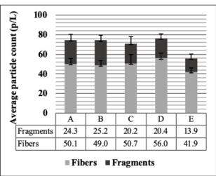
**Figure 4** Average particle count for  $\geq 20 \ \mu m$  (Fluorescent tagging)
