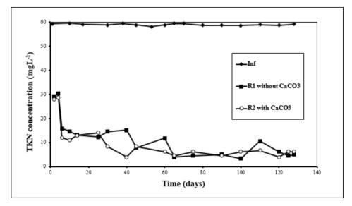
Figure 8 Influent and effluent concentration of TKN in SBR1 and SBR2.
