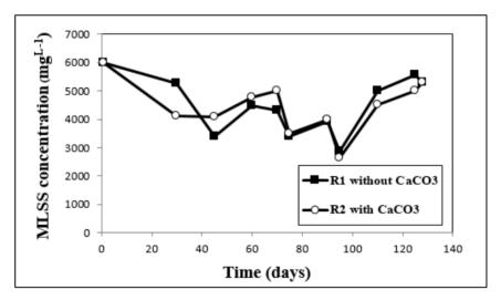
Figure 3 Variation of MLSS in SBR1 and SBR2 during 128 days of operation
