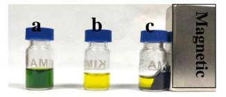
**Figure 3** Photography of clean- up performance by different DSPE adsorbents: (a) 1 mL Chinese kale extracts without DSPE clean-up; (b) 1 mL Chinese kale extracts with DSPE clean-up by 150 mg anh.MgSO<sub>4</sub>, 7.5 mg GCB 50 mg PSA and without Fe<sub>3</sub>O<sub>4</sub> MNPs; (c) 1 mL Chinese kale extracts with DSPE clean-up by 150 mg anh.MgSO<sub>4</sub>, 7.5 mg GCB and 50 mg PSA and 40 mg Fe<sub>3</sub>O<sub>4</sub> MNPs.
