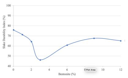
Figure 4 Relationship between slake durability index and bentonite dosage of composite clay liner
