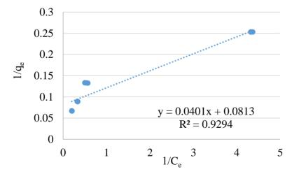
Figure 3 Langmuir isotherm plot for lead.
