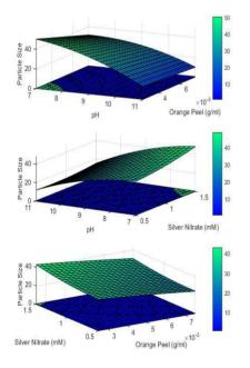
**Figure 7.** Surface plots showing AgNPs size as a function of orange peel conentration and pH (top), AgNO3 concentration and pH (middle), and orange peel extract
