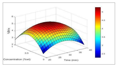
Figure 4 The 3D-graph showing the effect of concentration of solvent and treatment time on % brix at 1:15 solid to solvent ratio.
