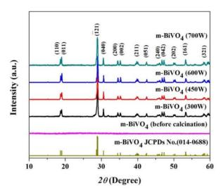
**Figure 1** XRD patterns of the un-calcined m-BiVO<sub>4</sub> powder and the m-BiVO4 powders synthesized using a combined microwave-calcination process.
