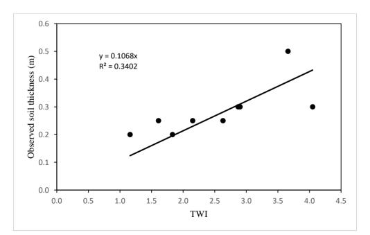
Figure 3 Linear relationship between TWI and soil thickness in Nam Hia creek catchment.
