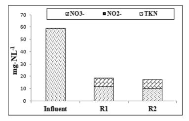
Figure 9 TKN effluent, NO<sub>2</sub><sup>-</sup> and NO<sub>3</sub><sup>-</sup> in SBR1 and SBR2.
