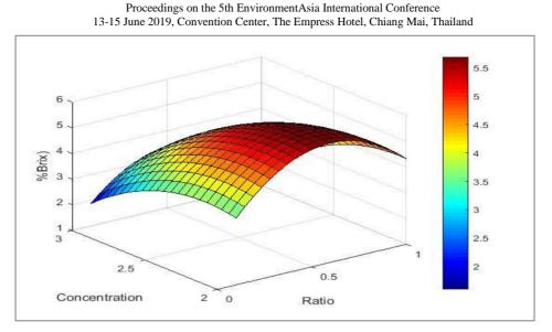
**Figure 3** The 3D-graph showing the effect of concentration of solvent and solid to solvent ratio on %brix at 30 minutes treatment time.
