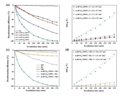
Figure 5. (a) Photocatalytic activities and (b) pseudo-first-order kinetics of the m-BiVO<sub>4</sub> photocatalysts for the photodegradation of MB under visible light irradiation. (c) and (d) A comparison of the photodegradation of BG, MO and MB in the presence of the m-BiVO<sub>4</sub> (700 W) photocatalyst under visible light irradiation.
