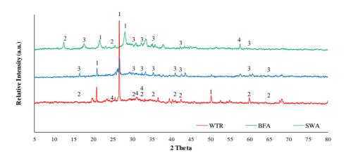
Figure 4 XRD of geopolymer at SiO<sub>2</sub>/Al<sub>2</sub>O<sub>3</sub> ratio of 3:1
