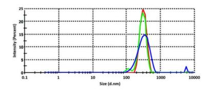
Figure 1 Particle size and size distribution of GO particles after size reduction
