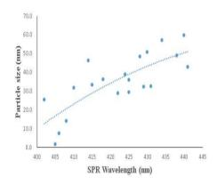
**Figure 8.** Relationship between the size of AgNPs and wavelength corresponding to peak surface plasmon resonance in UV-vis spectra.
