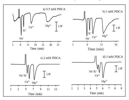
**Figure 4** The chromatogram of using various concentration of PDCA: a) 0.5 mM PDCA, b) 1 mM PDCA, c) 2 mM PDCA, and d) 3 mM PDCA using a column 1.5 m x 50  $\mu$ m, 13 layers of PBMA polymer, flow rate 0.6  $\mu$ L/min, AD7746 capacitance board as detector, injection volume 20 nL, mixed standards cations solution of 739  $\mu$ M Na<sup>+</sup>, 517  $\mu$ M K<sup>+</sup>, 1178  $\mu$ M Ca<sup>2+</sup>, and 2110  $\mu$ M Mg<sup>2+</sup>). The unit of capacitance value is femtofarad (fF).
