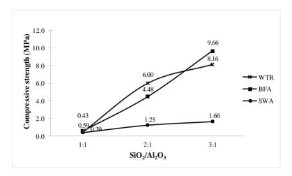
Figure 2 Strength of geopolymer at  $SiO_2/Al_2O_3 = 1:1 2:1$  and 3:1
