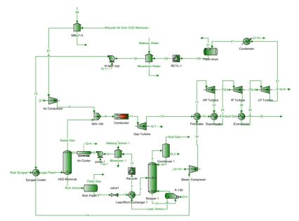
Figure 2. Schematic of the IGCC system with Promax® 4.0
