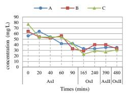
Figure 2 Cyclic profile of COD removal. (A) SRT 20 days; (B) SRT 25 days; (C) SRT 60 days. Ax is Anoxic condition, Ox is Oxic Conditio
