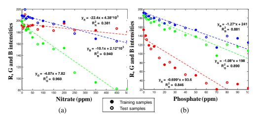
**Figure 3** Relationship between the concentrations of (a)  $NO_3^-$  and (b)  $PO_4^{3-}$  and the RGB intensities where the red, green and blue circle symbols represent each of the corresponding color intensities.
