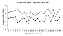
**Figure 1** Effect of removal the turbidity of raw water at adjustment the pH at 8.5
