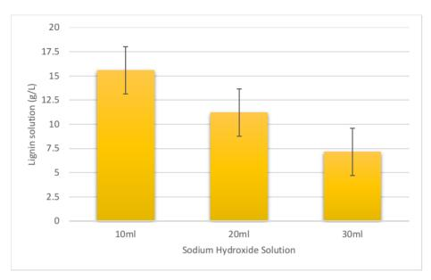
Figure 2 The amount of lignin solution from bagasse to sodium hydroxide solution ratios study.
